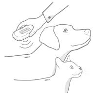
Press the button again, the reader scans for about 12 seconds after you press the button and maintain contact with the animal's body. Move the reader SLOWLY, following the recommended scanning patterns shown below.
